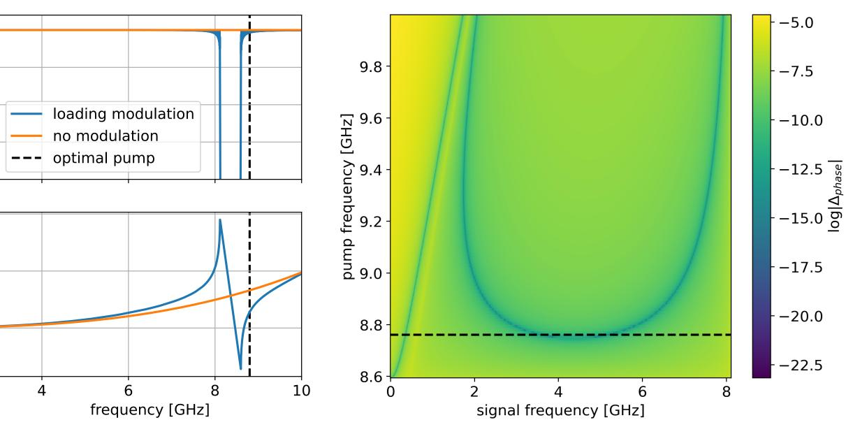
The cells are organized in supercells by modulating the loading periodically. Most common is step modulation.
