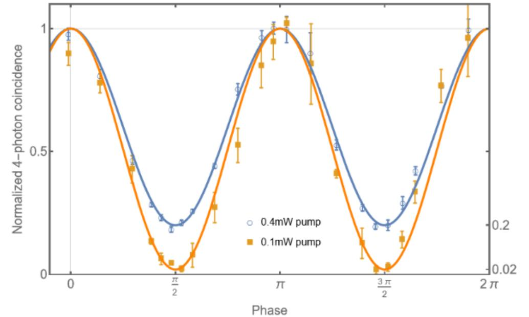
Fig. 4. HOM interference measured by 4-photon coincidence for the average pumping powers 0.1 and 0.4 mW per spiral, respectively. The measured visibility is 98% for the 0.1 mW pumping.
